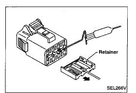
Some connectors do not have a notch above each terminal. To probe each terminal, remove the connector retainer to make contact space for probing.
