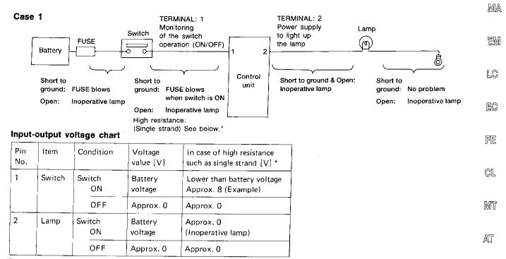
The voltage value is based on the body ground.
